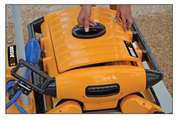
2. Remove the 2 filter bags from the robot.
