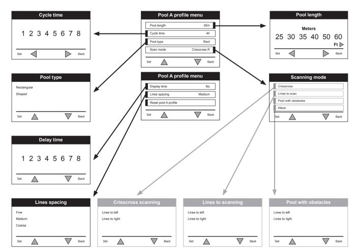
Figure 5: Manual Configuration of Pool Profiles
